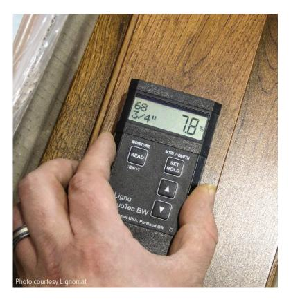
Make sure the sub floor and the concrete underneath are dry enough not to release extra moisture into the floor covering. This can cause problems within the first few months after the installation has been finished.
