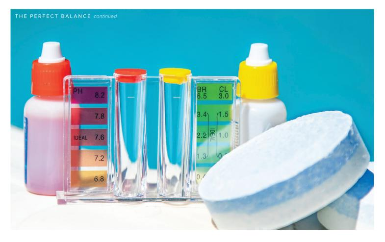
The concentration of HOCl is affected by both the pH and the CYA concentration. At low pH, chlorine is in its full active HOCl form. At high pH, chlorine is present as the less active hypochlorite ion. This situation is the primary reason pH must be controlled. Keeping the pH below 7.8 ensures an adequate HOCl concentration is maintained.
